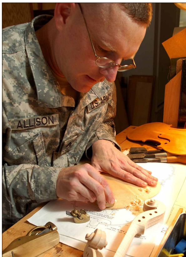
U.S. Army staff sergeant Geoffrey Allison uses a finger plane to shape a contour in the face piece of one of the violins he has in progress
